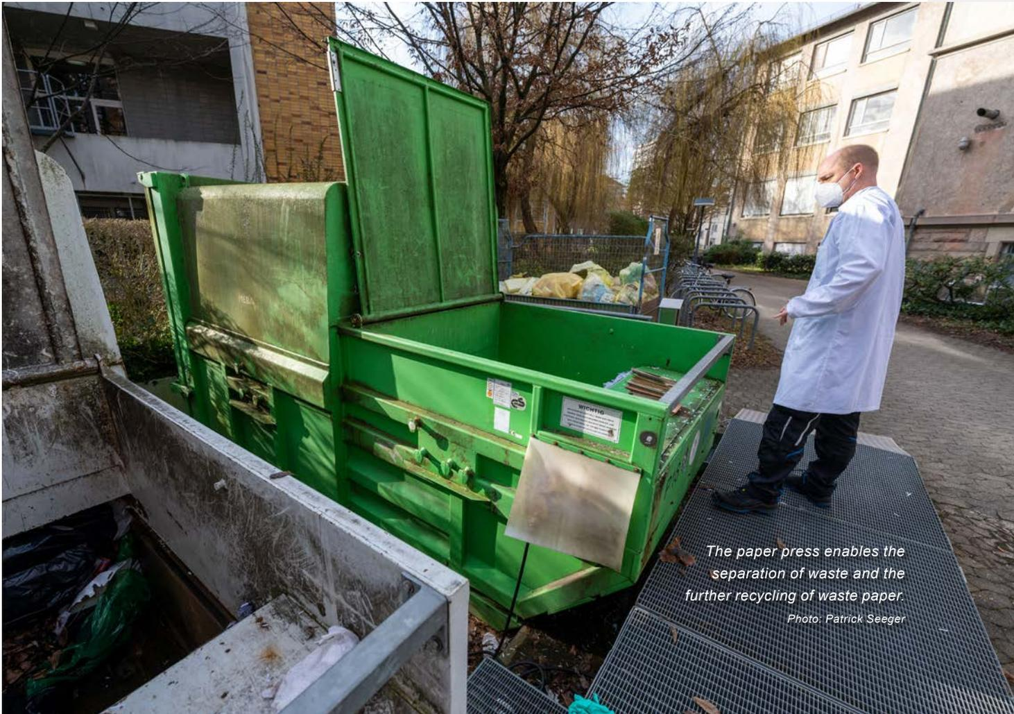
The paper press enables the separation of waste and the further recycling of waste paper.
