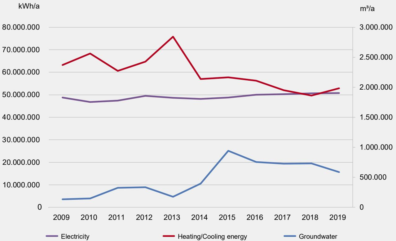
Energy used for heating and cooling increased significantly in 2019, exceeding electricity consumption. This rise occurred as the groundwater systems did not function properly during the survey period due to technical problems and construction work. As a result, less groundwater could
